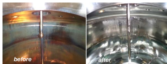
Fig. 3: Static, rotating and also orbital spray heads can wet all surfaces even in large autoclaves, preparation, production and storage vessels. (Author: Ateco)
