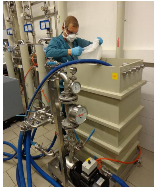
Fig. 5: When derouging with DIRUPURE, water for cleaning is heated to the required temperature in an external tank, for example, and the liquid or solid components are added and dissolved. (Author: Ateco)
