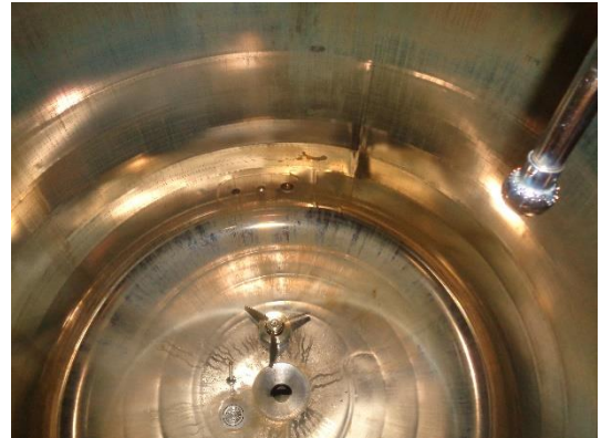
Fig. 1: The chromium content of the protective layer is already depleted in pure water at temperatures above 40 °C. The increased iron content then forms rouge. (Author: Ateco)
