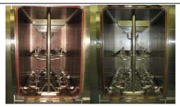
The new agent allows both flooding and spraying processes and circulation through the pipes. Autoclaves can be cleaned quickly and safely. 1a) autoclave before cleaning, 1b) autoclave three months after derouging, still perfect surface through the newly created passive layer.
