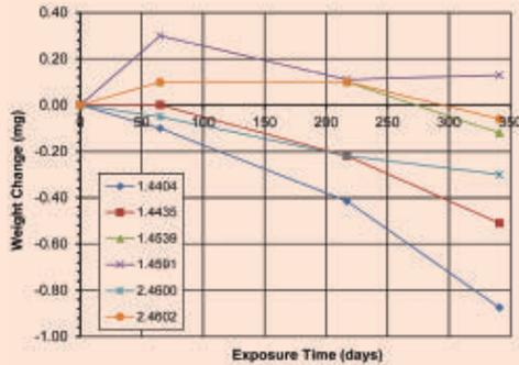
**Figure 4** Material-specific corrosion rates for the maximum exposure time of 354 days
