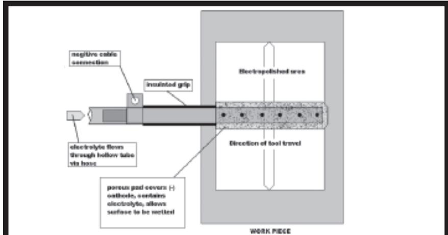
Figure 2. Illustration of tool used for manual electropolishing (in situ electropolishing).
