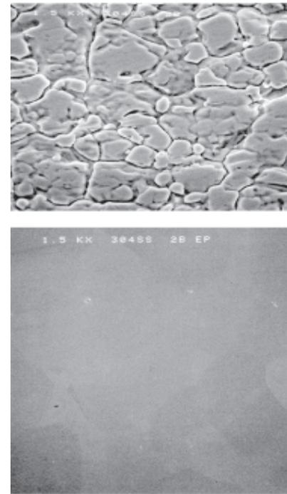
Figure 4. 2B sheet, mill finish, 10 Ra μin (top). 2B sheet after electropolishing, 7 Ra μin (bottom). Both surface at 1,500 X. Electropolishing leaves little or no grain boundaries or surface imperfections.
