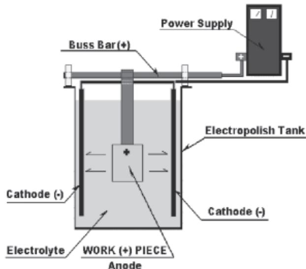
Figure 1. A simple electropolishing set-up for items that can be processed in a tank.
