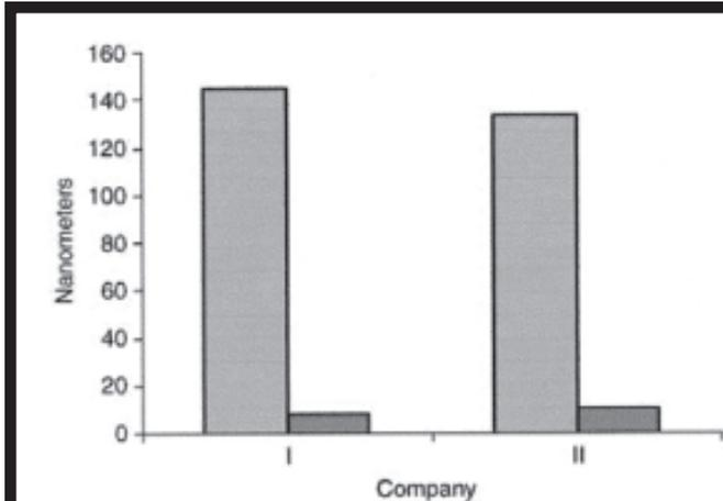
Figure 7. Comparison of surface roughness on stainless steel samples from two manufacturers. The average roughness for the electropolished samples (dark bars) was reduced from the control samples (light bars).
