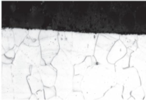
Figure 5. Mechanically polished surface showing a cold-worked surface approximately 0.0003-in deep (top). Surface layer with cold-worked surface layer removed after electropolishing (bottom). Illustration of cold-worked surface layer resulting from mechanically polishing and removal by electropolishing.
