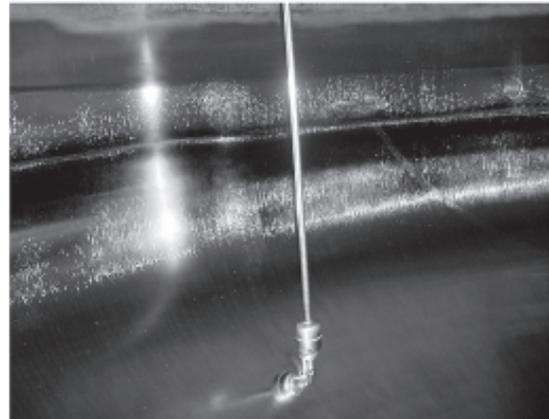
Figure 6. Electropolished band remained rough free while mechanically polished surfaces developed rouge (top), as while as the bottom head that was electropolished remained free of rouge (bottom).
