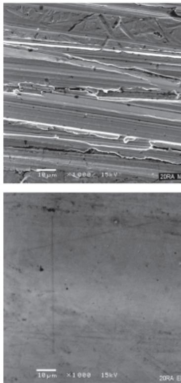
Figure 3. Mechanically polished surface, 20 Ra μin (top). Electropolished surface, 20 Ra μin (bottom). Surfaces shown at 1,000 X with same Ra μin.
