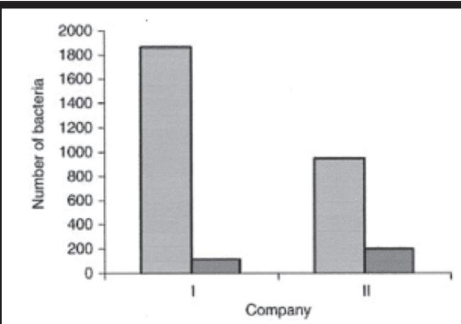
Figure 8. Comparison of bacterial attachment with stainless steel samples from two manufacturers. The numbers of attached bacteria on electropolished samples (dark bars) were significantly reduced from the control samples (light bars).
