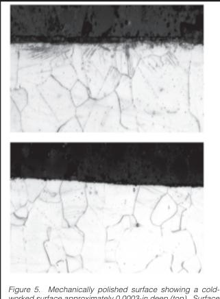
Figure 5. Mechanically polished surface showing a coldworked surface approximately 0.0003-in deep (top). Surface layer with cold-worked surface layer removed after electropolishing (bottom). Illustration of cold-worked surface layer resulting from mechanically polishing and removal by
