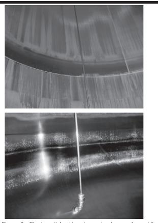
Figure 6. Electropolished band remained rouge free while mechanically polished surfaces developed rouge (top), as while as the bottom head that was electropolished remained free of rouge (bottom).
