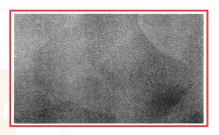
No 2B Mill Finish after electropolishing. Note that grain boundaries have been removed, eliminating sites for contamination to be retained.
